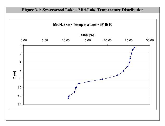
Swartswood Lake was strongly thermally stratified during the 18 August 2010 event as indicated in figure 3.1. The epilimnion extended from the surface to 4 m with the thermocline extending to 9 m.
