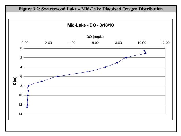
Dissolved oxygen concentrations varied significantly throughout the water column due to thermal stratification and varying rates of production versus respiration. DO concentrations were supersaturated in the epilimnion and declined to anoxic conditions at depths of 8 m and greater. DO concentrations were greater than Princeton Hydro's recommended threshold of 4.0 mg/L throughout the upper 5 m of the water column.
