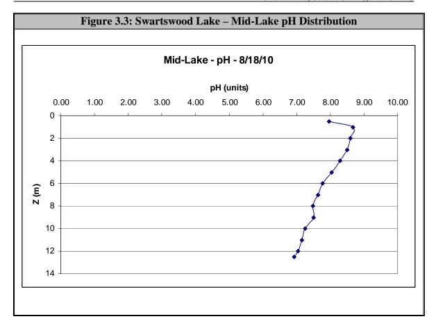
pH values throughout the water column showed normal spatial variation as reflected by varying rates of photosynthesis versus respiration. Overall, pH values were within an appropriate range for the support of aquatic life and were of no cause for concern.
