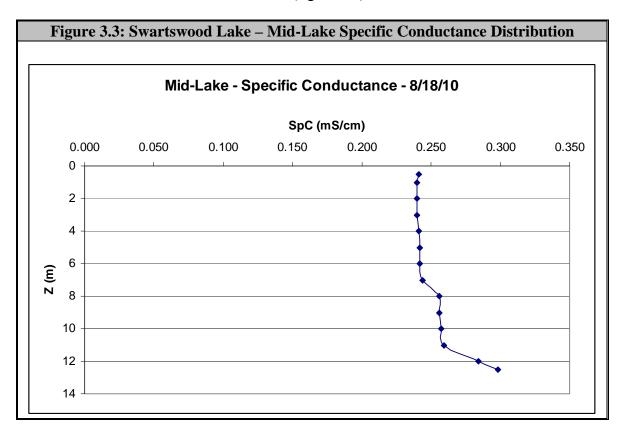
Specific conductance values were homogenous throughout the upper 7 m and then increased throughout the hypolimnion as a result of anoxia and associated reducing conditions at the sediments which served to release ionic constituents into the overlying water.
